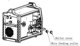
9.1 open the door of the machine shell. Please remove the wire first if there is still wire on the wire feeder;
